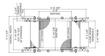
All standard crossover stairs (10", 19-1/2", 29", 38-1/2", 48" and 65" clearances) have 2'-6" wide stair treads and an overall width of 3' 3-3/4".
